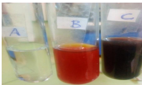
Fig. 12. Color change of the leaf extract: A) 4mM AgNO 3 solution (colorless) B) aqueous extract of Coffea arabica leaves (yellowish brown) C) synthesized AgNO 3 (deep brown)
