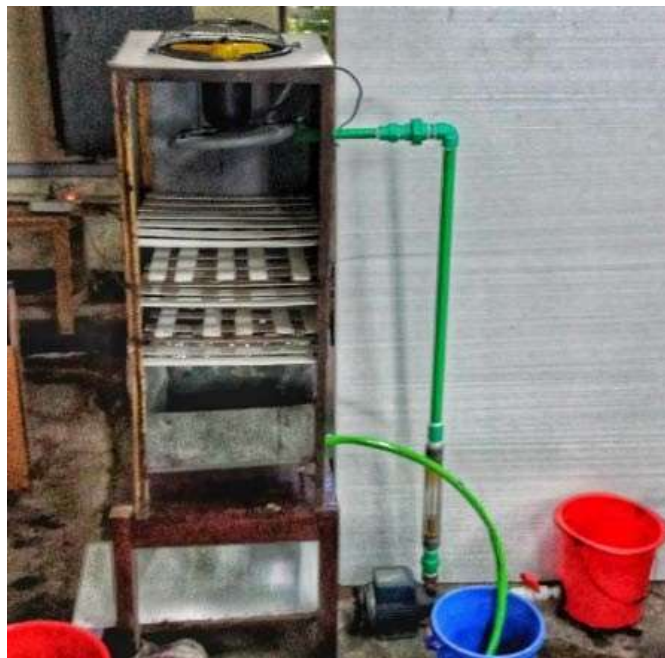
Fig. 5. Cooling tower with regular-shaped splash fills
