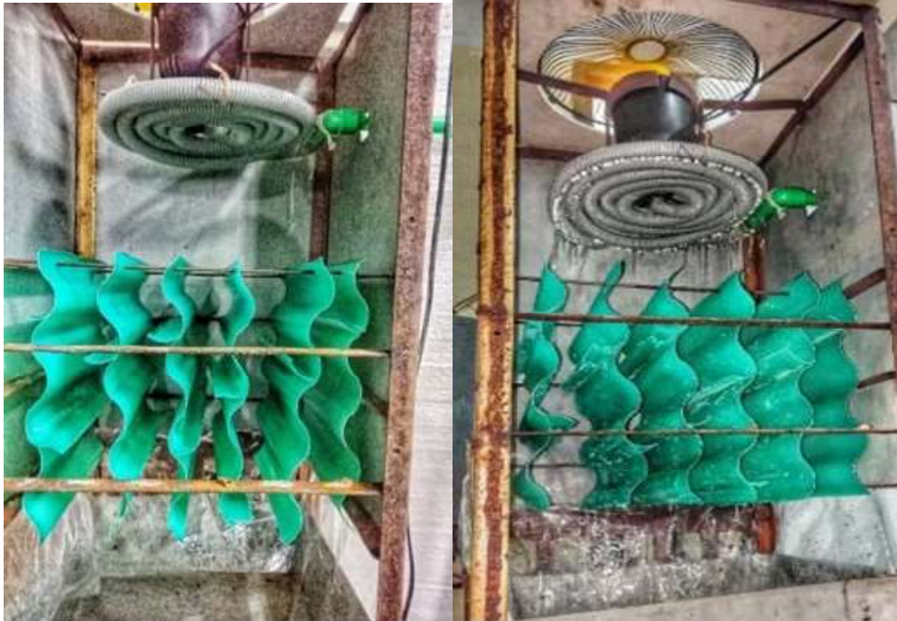
Fig. 8. Cooling tower with film fills with ripple plates
