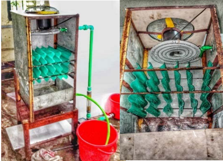
Fig. 6. Cooling tower with regular-shaped film fills
