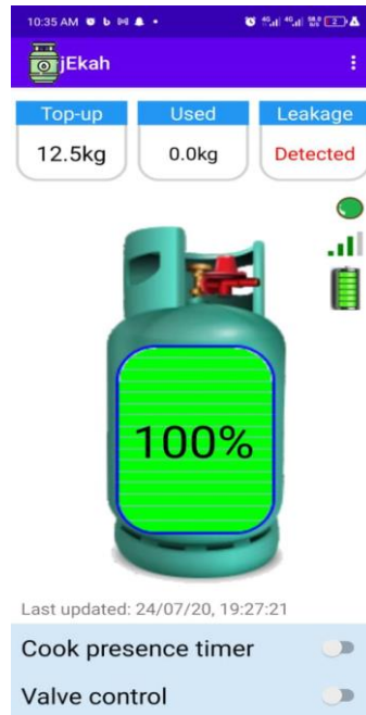
Fig. 11. Gas leakage notification via mobile app
