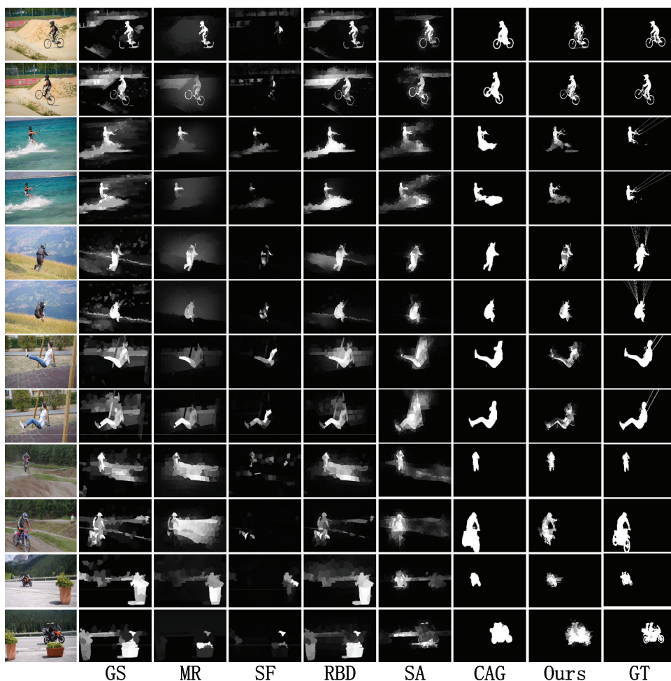
Figure 9. Experimental results of FMP and other six advanced object saliency detection algorithms results in the DAVIS and SegTrackv2 datasets.
