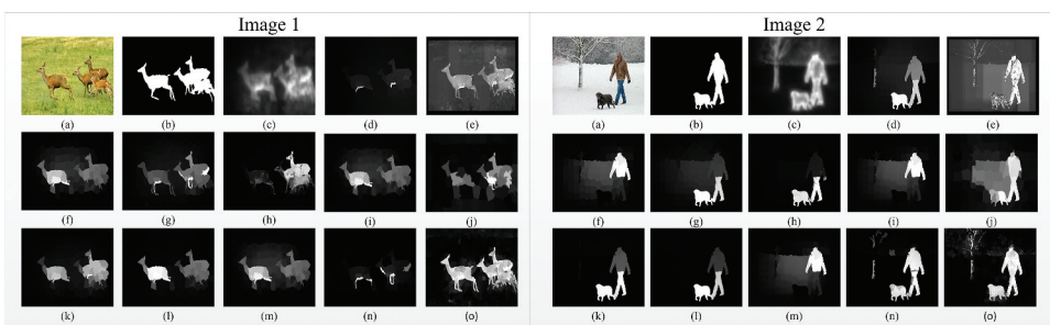
Figure 5. Qualitative analysis of the proposed algorithm on HKUIS dataset compared to other salient object detection techniques (a)Original Image (b)Groundtruth (c)CA (d)GR (e)SEG (f)MR (g)MC (h)LPS (i)RR (j)LGF (k)DPSG (l)NCUT (m)RCRR (n)SMD (o)LGSD-DCPCNN.
