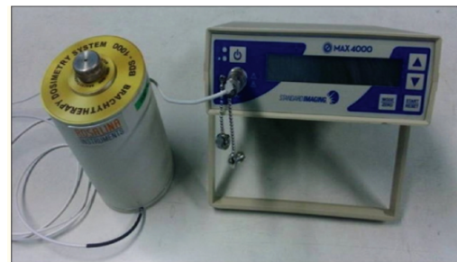
Fig. 4. BDS 1000 well-type ionization chamber with the standard imaging MAX 4000 electrometer [16]
