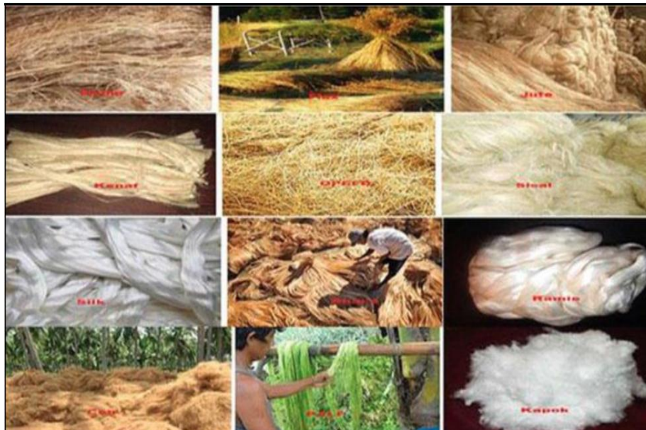
Fig. 2. Different natural fibers are frequently included as reinforcements in polymer composites [13]
