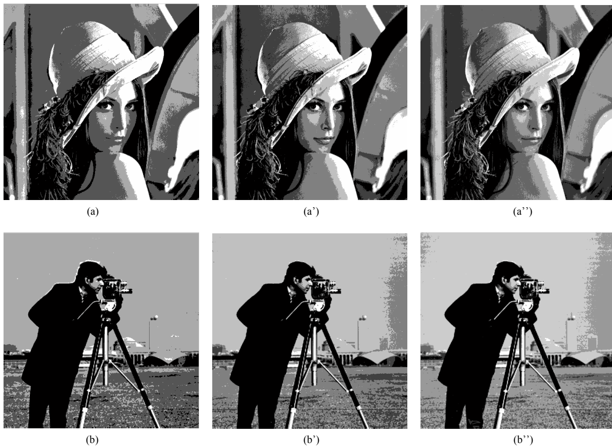
Figure 2. Thresholded images obtained by Kapur-PSO method ((a), (b) represents 3-level thresholding, (a'), (b') represents 4-level thresholding, (a''), (b'') represents 5-level thresholding)
