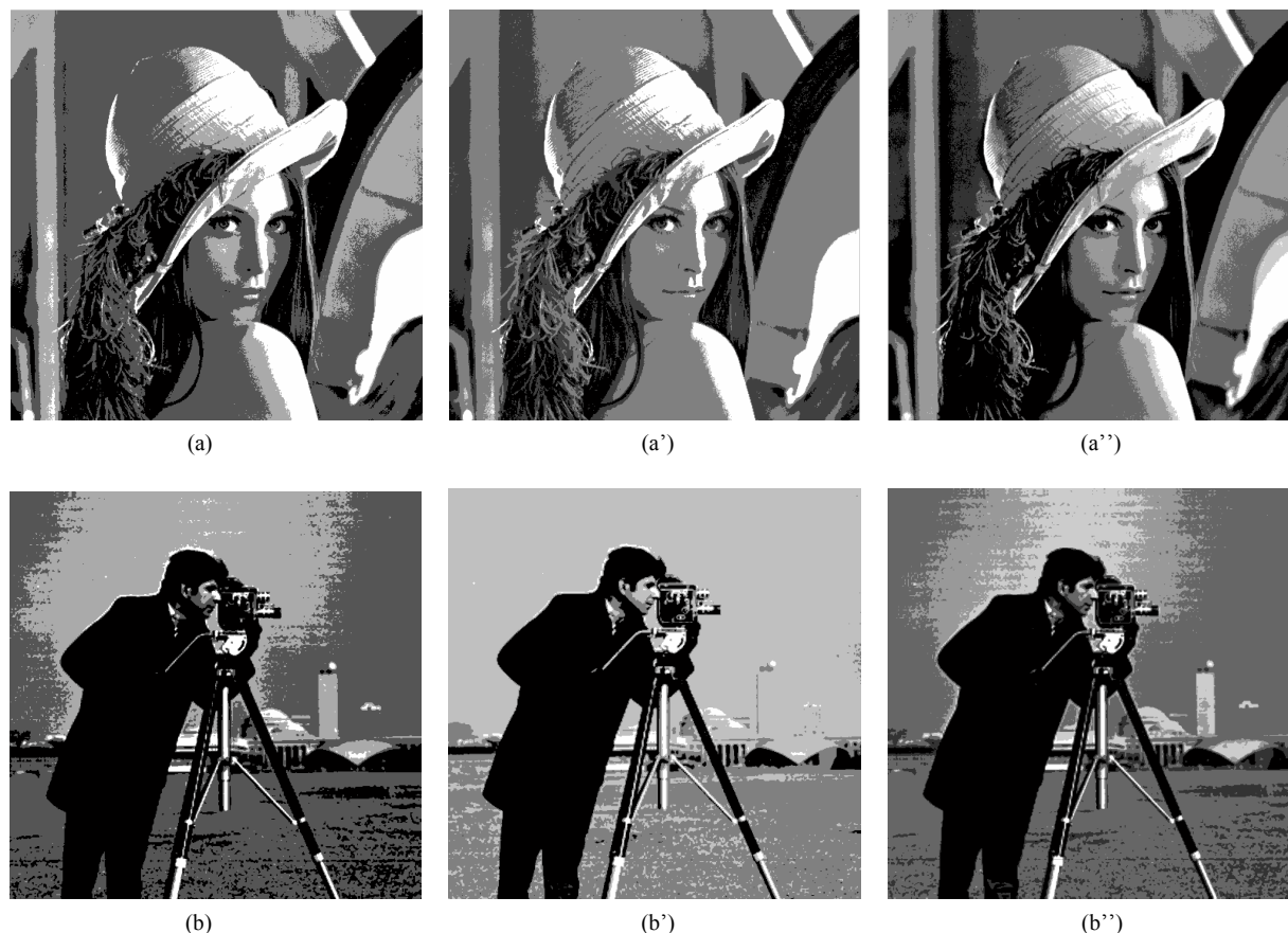
Figure 3. Thresholded images obtained by Otsu-PSO method ((a), (b) represents 3-level thresholding, (a'), (b') represents 4-level thresholding, (a''), (b'') represents 5-level thresholding)
